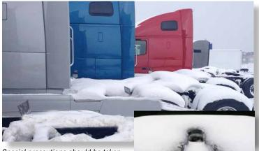
Special precautions should be taken during extreme cold weather to ensure that the fifth wheel locking mechanism operates freely. At low temperatures ice and sludge can build up, and lubricants can become
