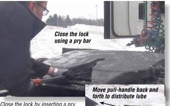
Close the lock by inserting a pry bar into the throat of the fifth wheel to activate the trigger mechanism. Keep hands out of the fifth wheel throat. Move the handle back and forth several times without fully engaging the lock to distribute the fresh lubricant.
